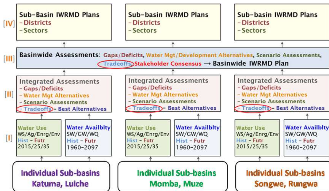
Figure 2.1: IWRMD Plan Preparation Approach Intended to (a) Integrate Regional Resources and Sectoral Interests and (b) Develop Stakeholder Consensus on a Shared Vision Basin Plan.
